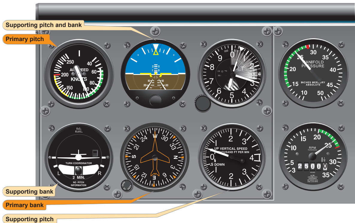
Figure 7-26. Stabilized climb at constant airspeed.
