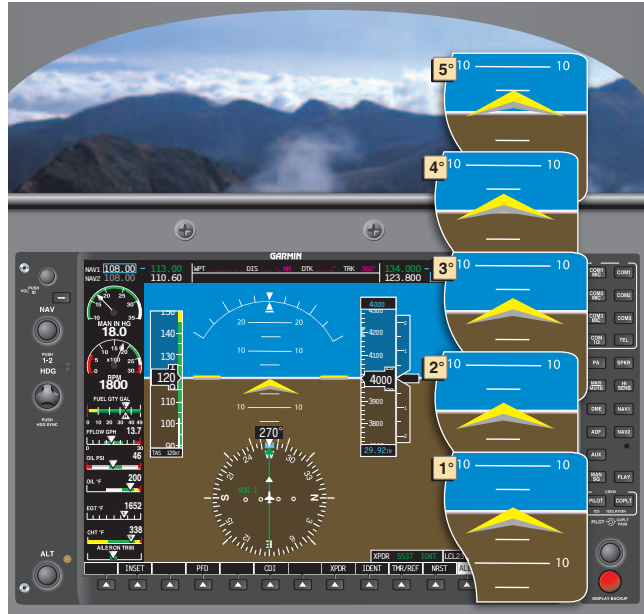
Figure 7-49. Various pitch attitudes (right), aircraft shown in level flight.
