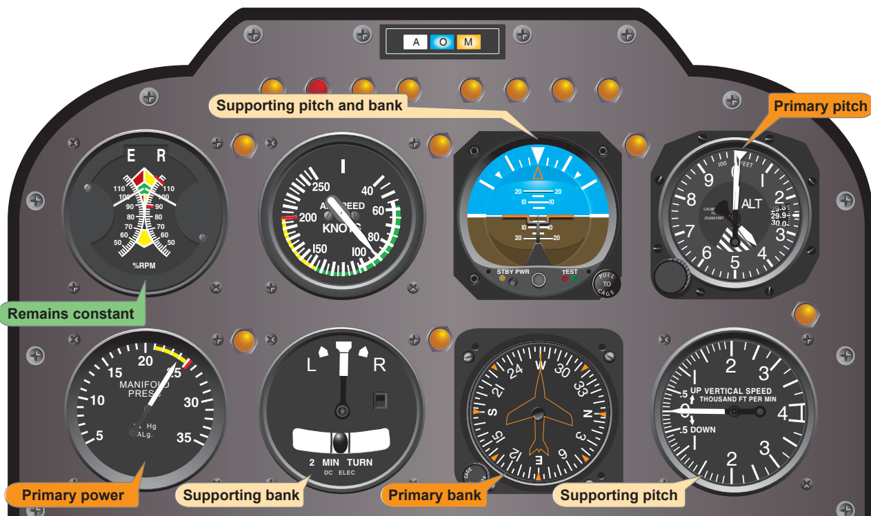
Figure 8-9. Flight instrument indications in straight-and-level flight at normal cruise speed.
