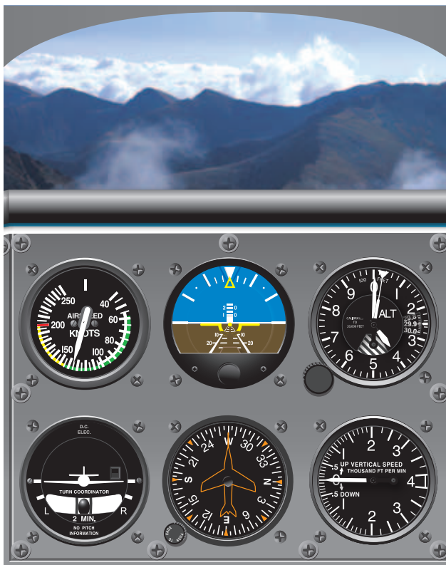
Figure 7-2. Pitch attitude and airspeed in level flight, fast cruise speed.
