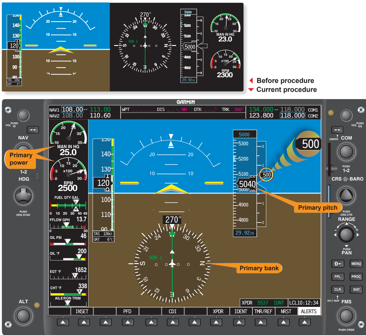
Figure 7-63. Constant airspeed climb from cruise airspeed.
