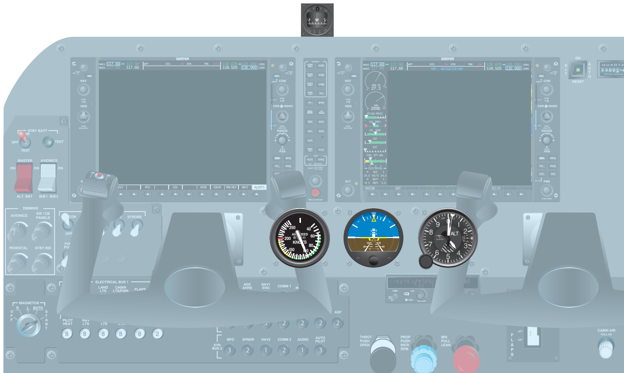
Figure 6-24. Emergency back-up of the airspeed indicator, attitude indicator, and altitude indicator.
