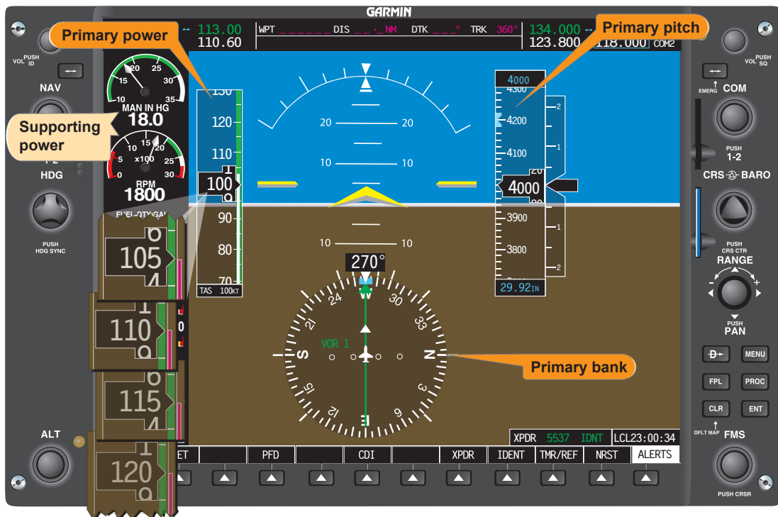
Figure 7-59. Straight-and-level flight (reduced airspeed stabilized).
