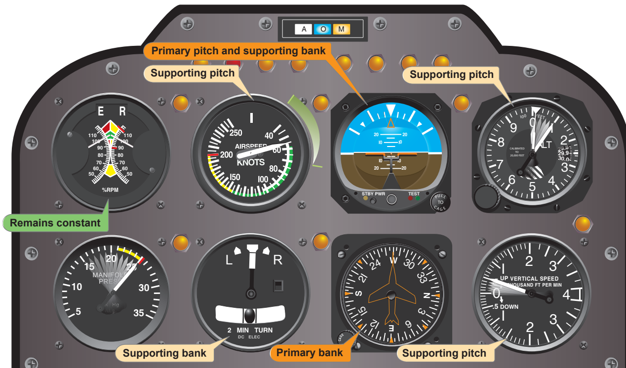
Figure 8-16. Flight instrument indications during an instrument takeoff.
