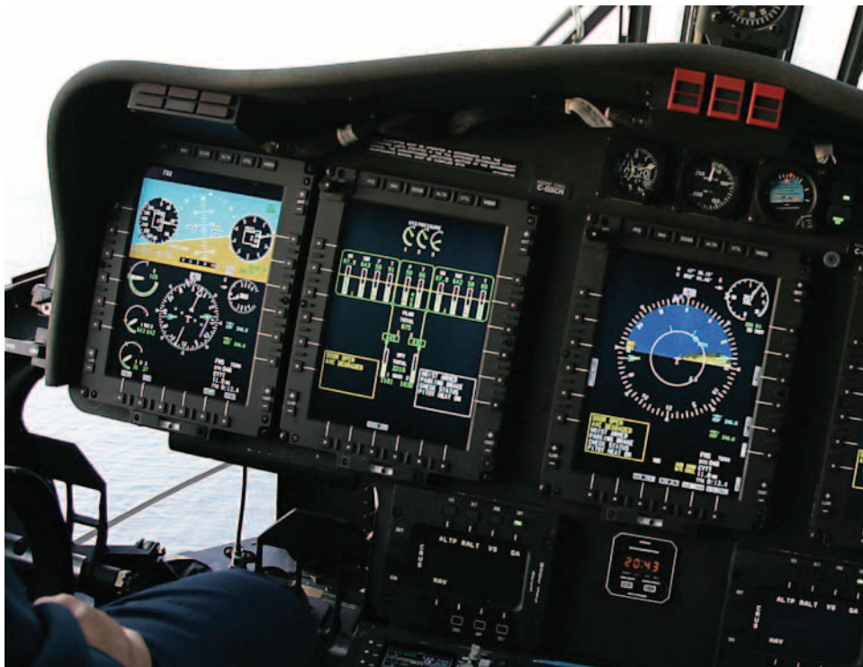
Figure 8-20. MFD display of aircraft systems.
