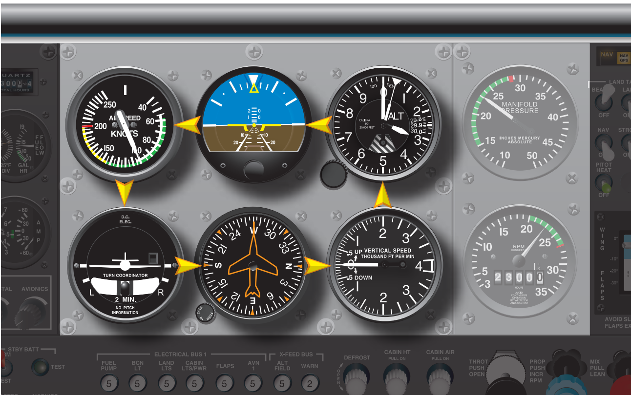
Figure 6-19. Rectangular cross-check.
