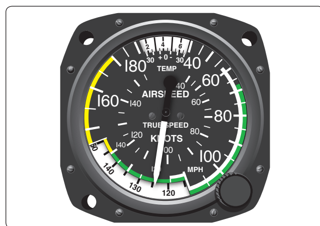
Figure 5-12. A true ASI allows the pilot to correct IAS for nonstandard temperature and pressure.
