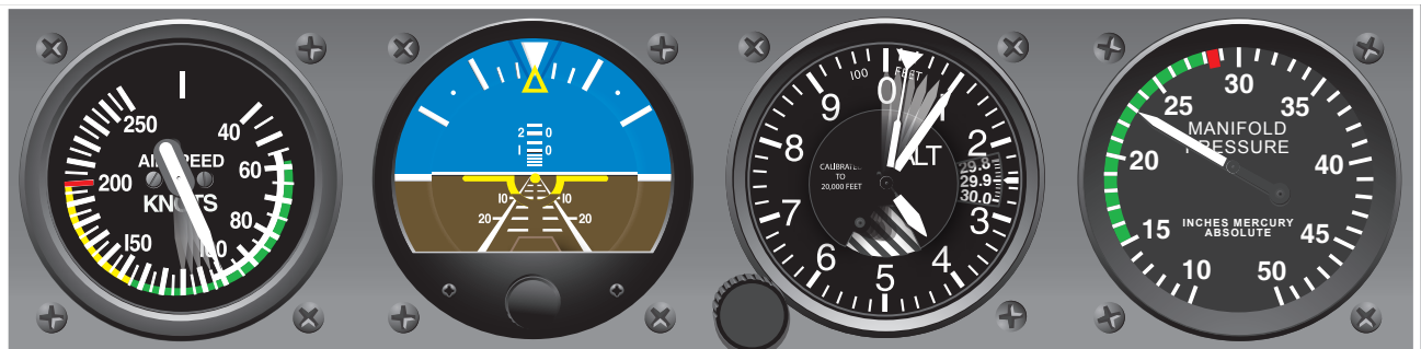
Figure 7-20. Airspeed low and altitude high—lower pitch.
