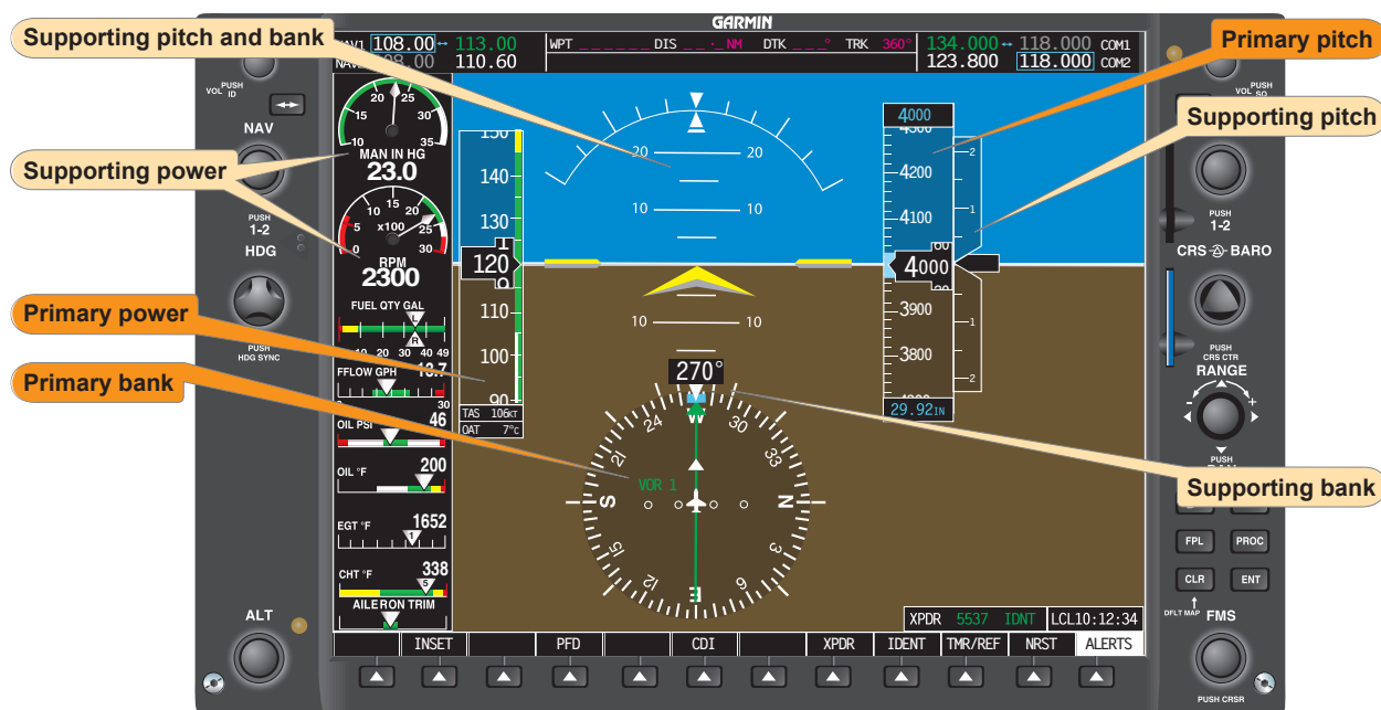
Figure 7-57. Straight-and-level flight (normal cruising speed).
