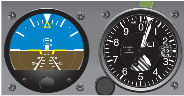
Figure 7-9. Altitude error, less than 100 feet.
