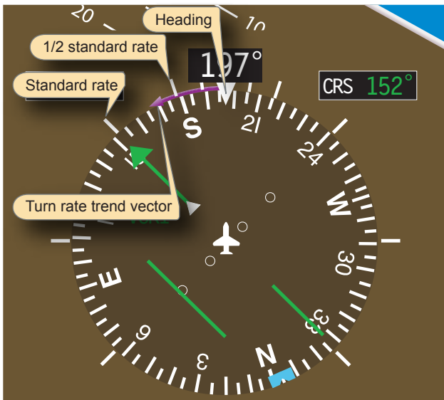
Figure 6-39. HSI indicator (enlargement).
