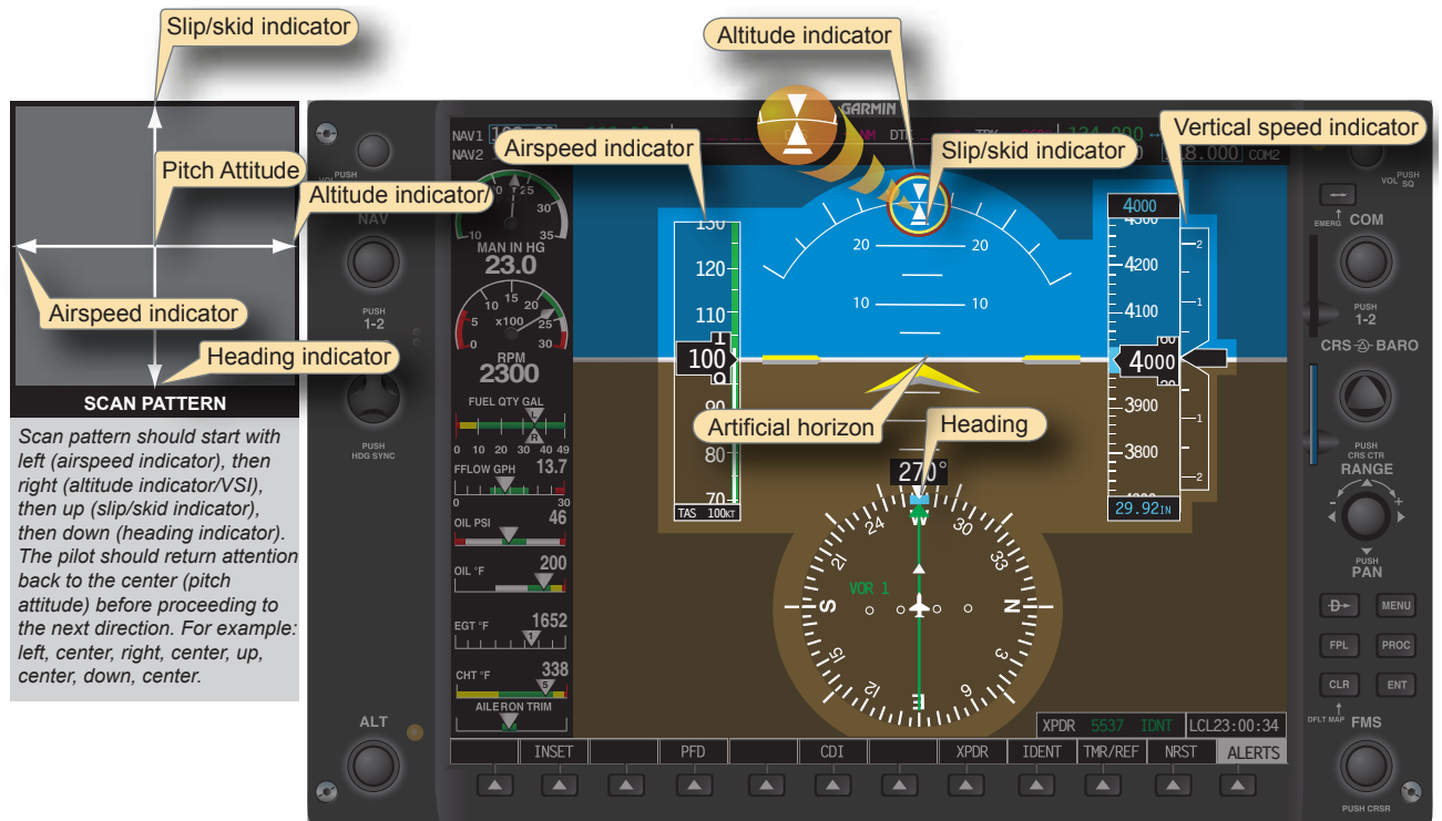
Figure 6-33. Selected radial cross-check.
