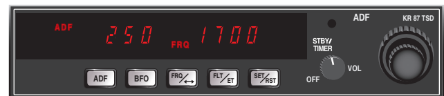
Figure 9-2. ADF indicator instrument and receiver.
