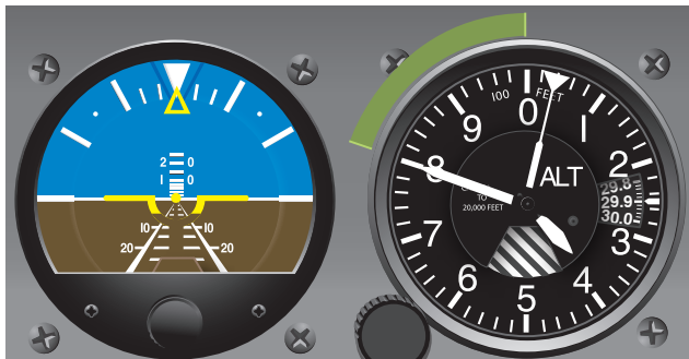
Figure 7-11. Altitude error, greater than 100 feet.
