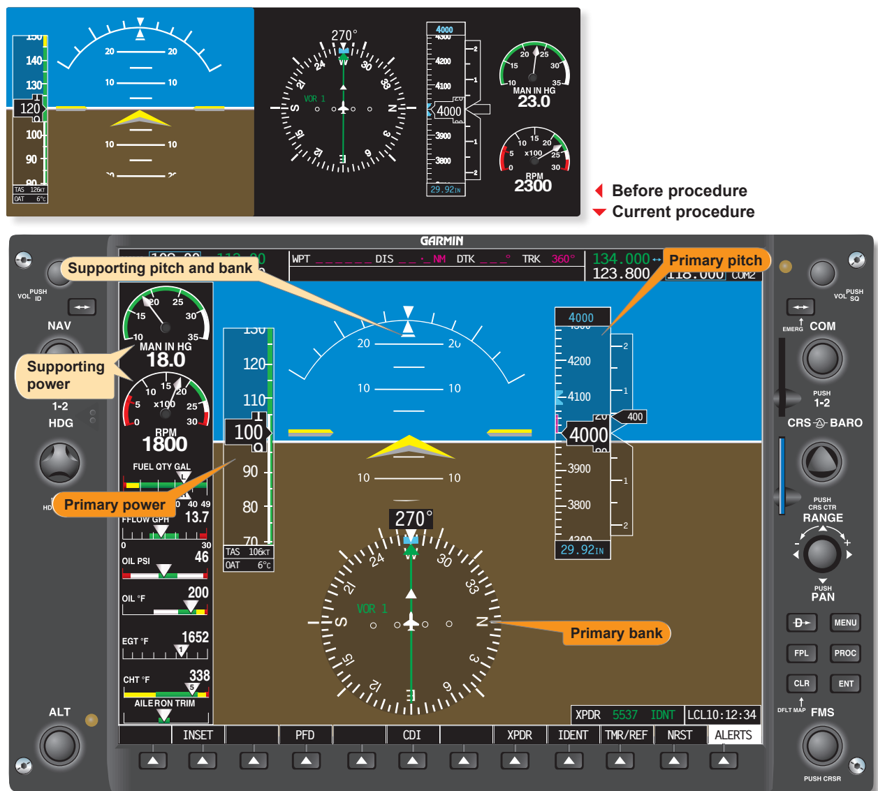
Figure 7-64. Constant airspeed climb from established airspeed.
