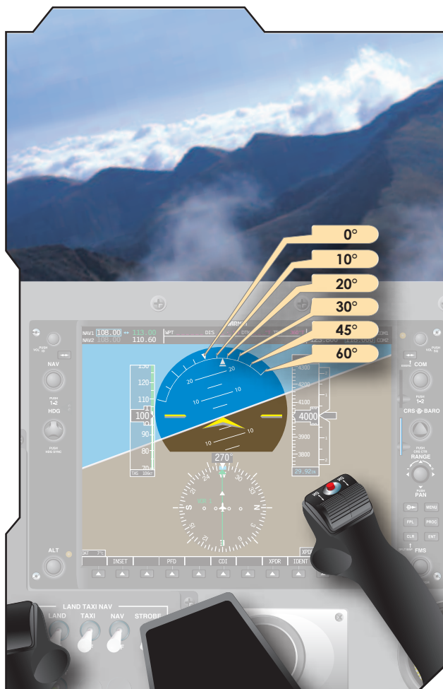
Figure 6-29. Bank indicator index lines.
