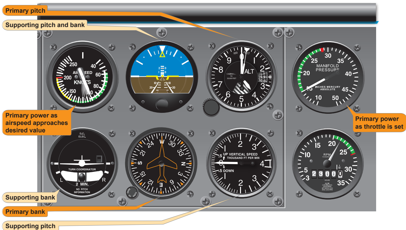
Figure 7-23. Straight-and-level flight (airspeed decreasing).
