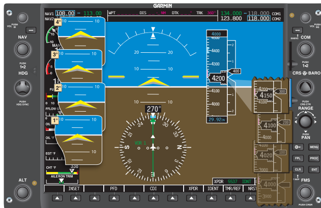
Figure 7-50. Pitch indications for various attitudes (1° through 5°).
