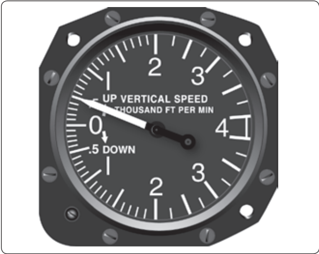
Figure 5-10. Rate of climb or descent in thousands of feet per minute.
