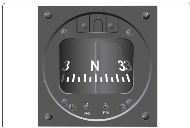
Figure 5-16. A magnetic compass. The vertical line is called the lubber line.
