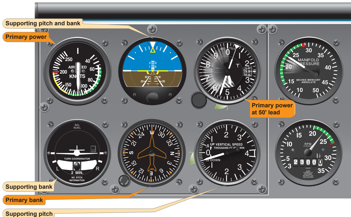
Figure 7-32. Level off at descent airspeed.
