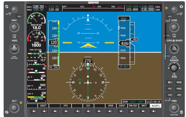
Figure 7-51. Pitch illustrated at 10°.
