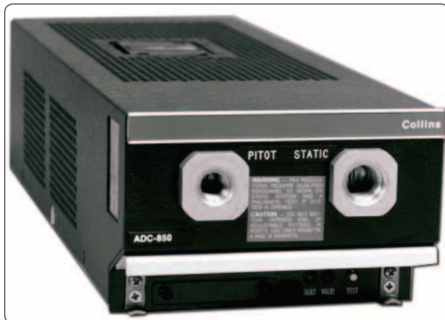
Figure 5-37. Air data computer (Collins).
