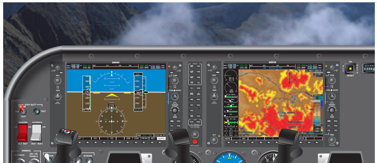
Figure 7-48. Pitch attitude decreasing and airspeed increasing—indicates need to increase pitch.
