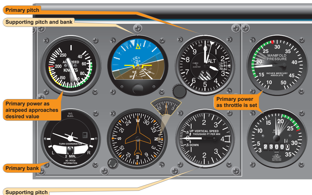
Figure 7-38. Change of airspeed during turn.
