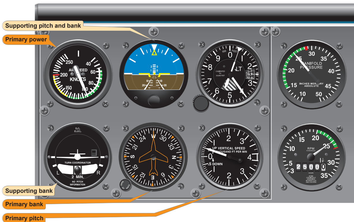
Figure 7-27. Stabilized climb at constant rate.
