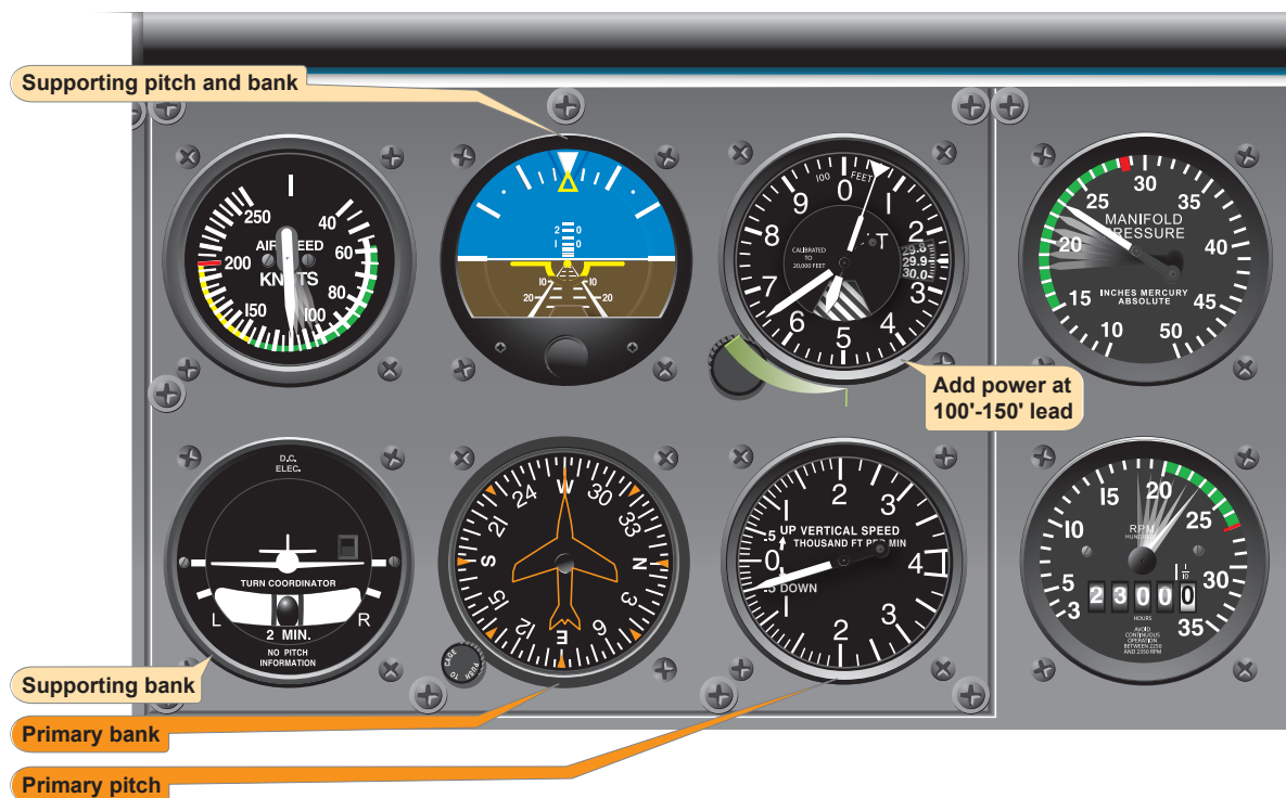
Figure 7-31. Level off airspeed higher than descent airspeed.
