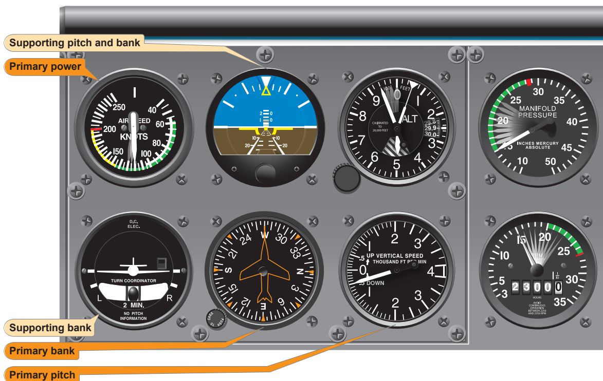
Figure 7-30. Constant airspeed descent, airspeed high—reduce power.
