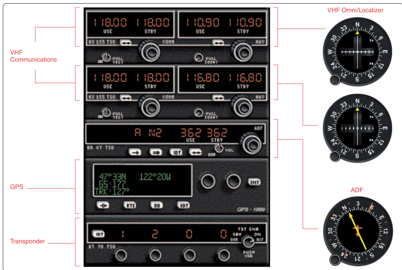
Figure 2-1. Typical navigation/communication installation.
