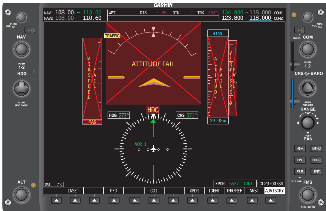
Figure 7-74. AHRS ADC failure.
