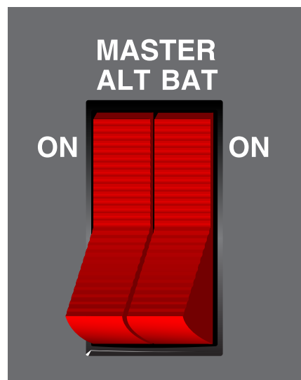
Figure 11-5. Double rocker switch seen on many aircraft.
