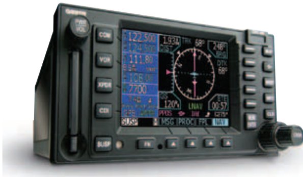
Figure 9-26. A typical example (GNS 480) of a stand-alone GPS receiver and display.
