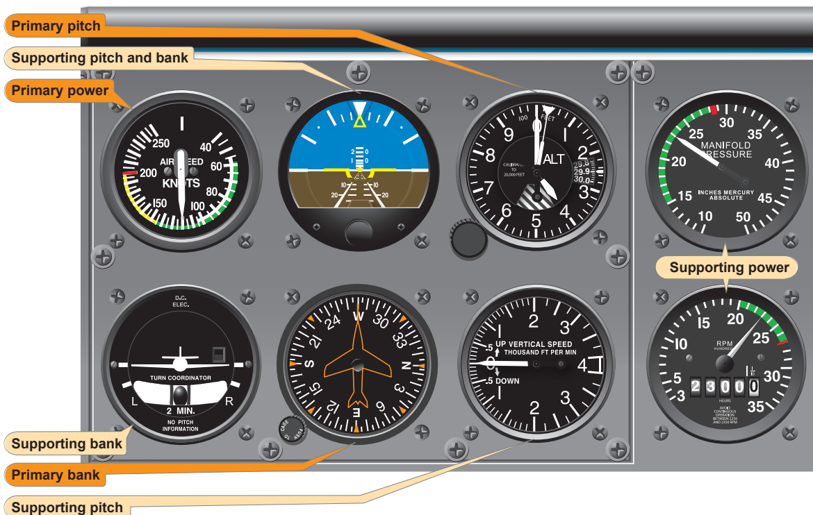
Figure 7-22. Straight-and-level flight (normal cruising speed).
