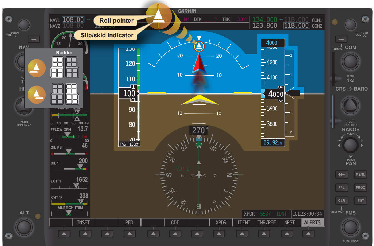
Figure 6-34. Roll pointer and slip/skid indicator.
