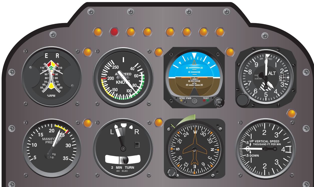
Figure 8-8. Flight instrument indications in straight-and-level flight with power decreasing.
