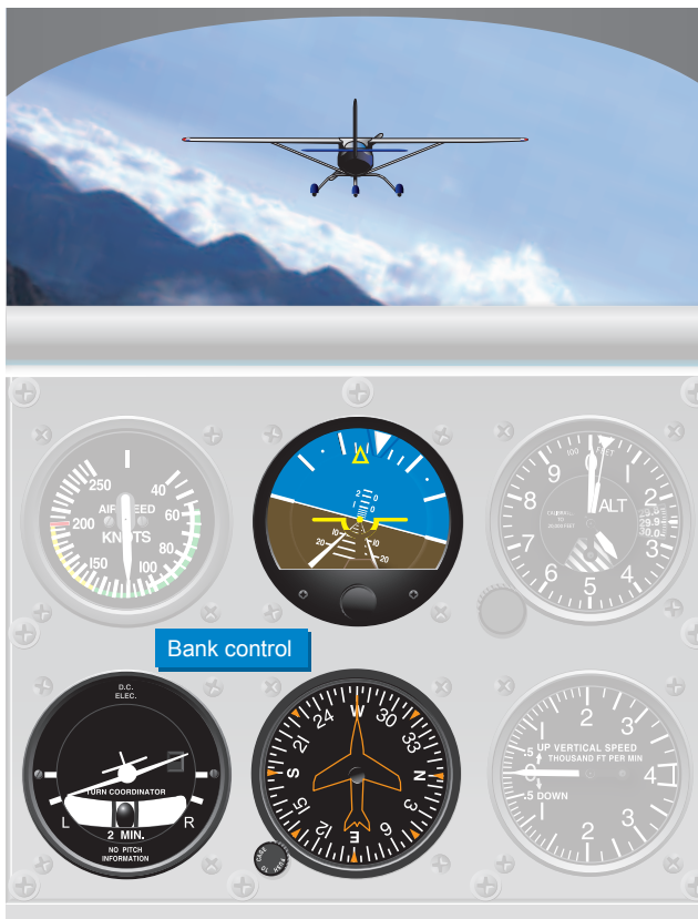
Figure 7-16. Instruments used for bank control.
