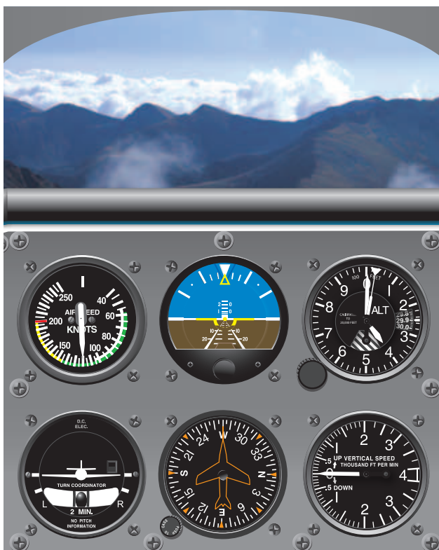
Figure 7-3. Pitch attitude and airspeed in level flight, normal cruise speed.
