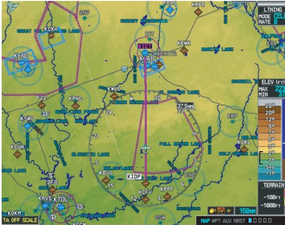
Figure 8-19. MFD display of a moving map.
