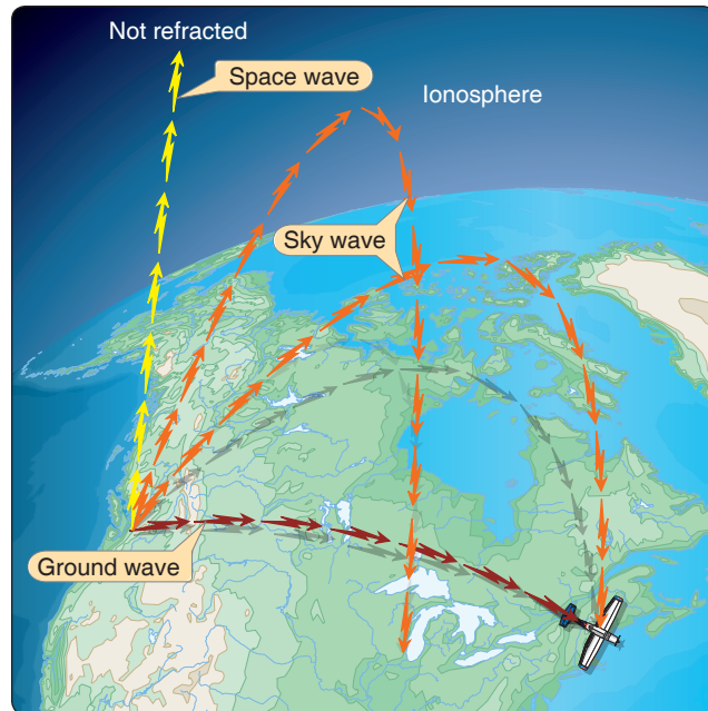
Figure 9-1. Ground, space, and sky wave propagation.
