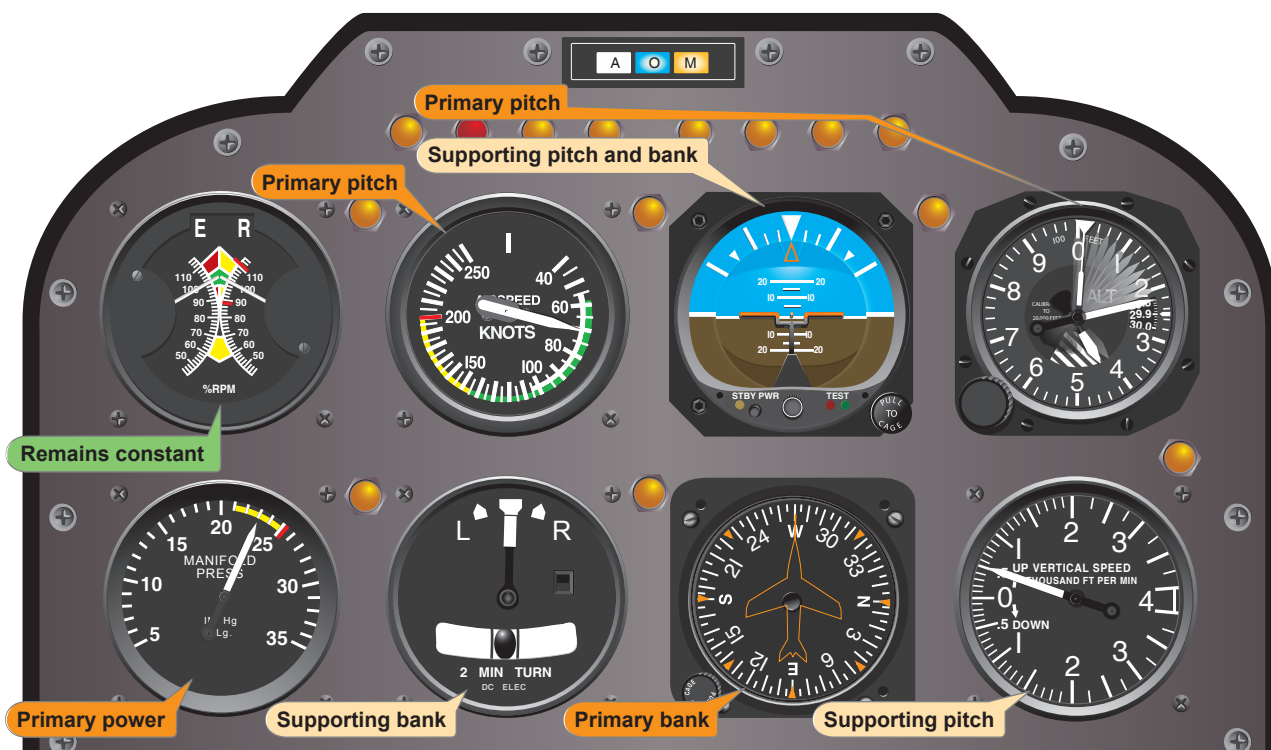
Figure 8-12. Flight instrument indications in a stabilized constant-airspeed climb.
