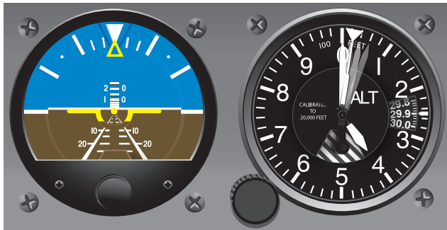
Figure 7-10. Pitch correction, less than 100 feet—one-half bar low to correct altitude error.
