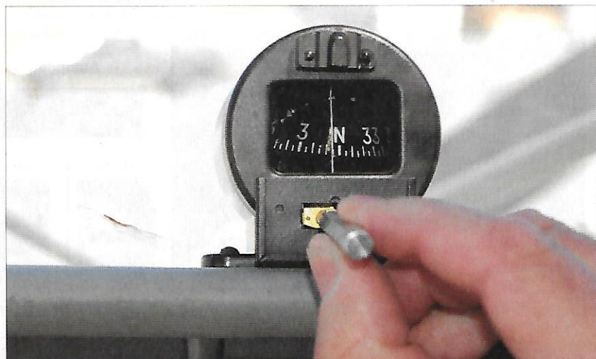
The owner of this plane uses a non-magnetic aluminum screwdriver to adjust his compass. There are two adjustment screws: one for north-south and one for east-west.
