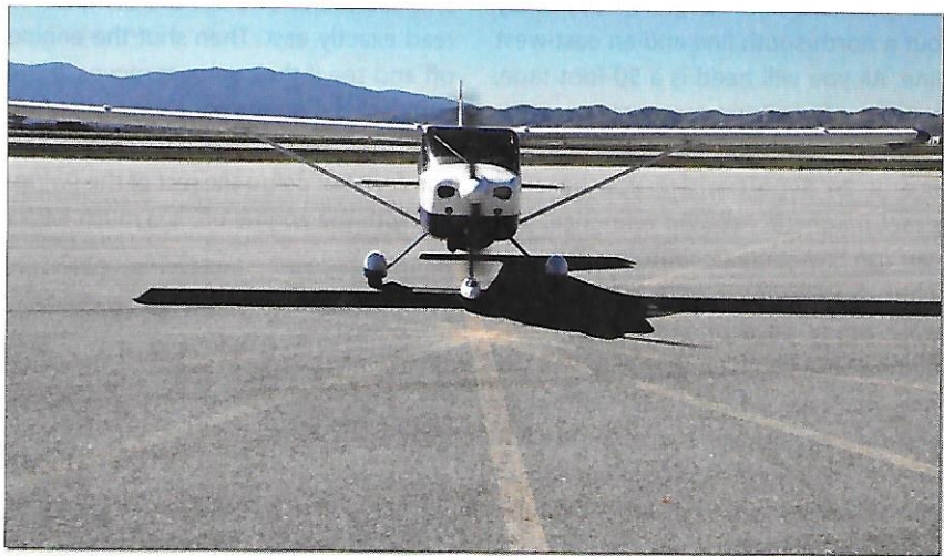
Align your plane with the compass rose as closely as possible. You will need to keep your engine running if it affects your compass readings.
