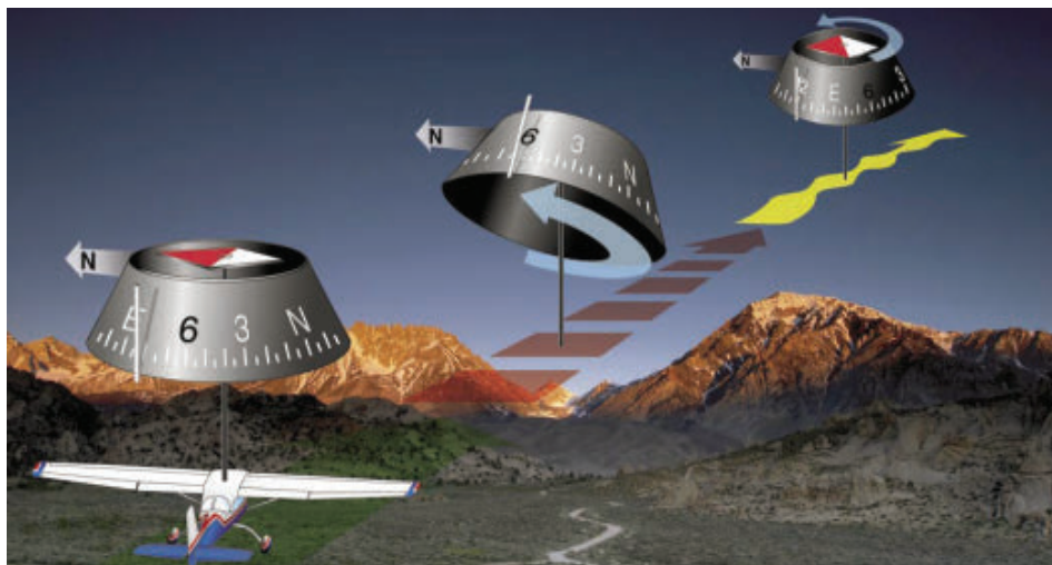
When accelerating on an east/west heading the compass needle points slightly north; when decelerating it will point slightly south.
