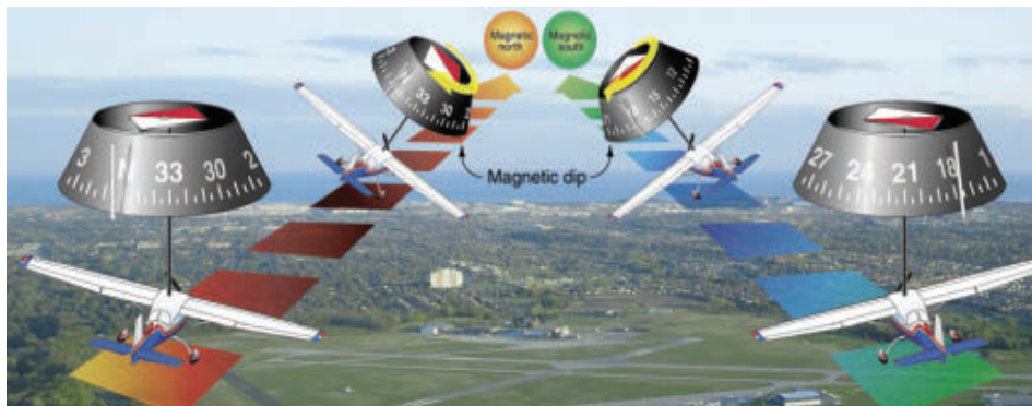
The compass indication will lag when initiating a turn from a northern heading to the east. Turning from a southern heading to the east, the compass indication will lead the turn.
