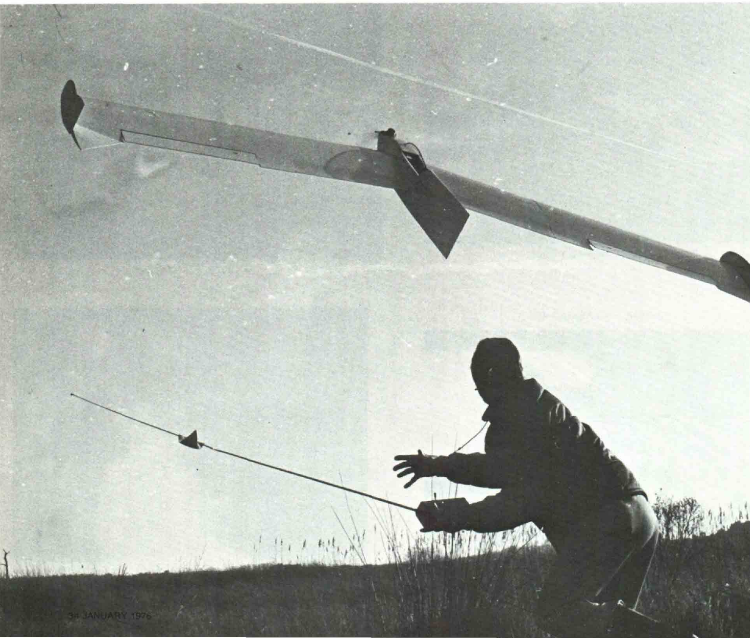
FIGURE 9 — First test flight of Woody Blanchard's .3 scale Kasper BKB 1A. Surprisingly, it recovered from this bad first launch which was the result of too much up-elevon trim.
