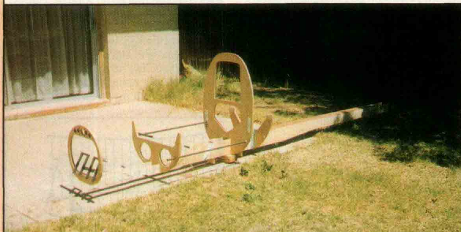
Fuselage skeleton consists of 4 plywood bulkheads sitting on a wood/plywood boom.
