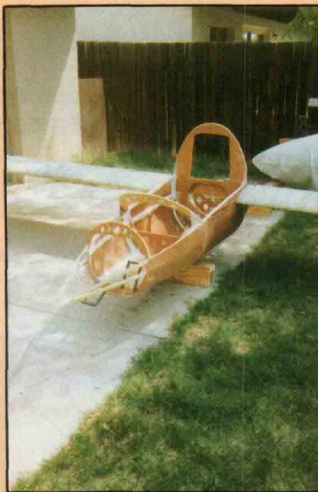
Fuselage pod is covered with plywood, followed by fiberglass.
