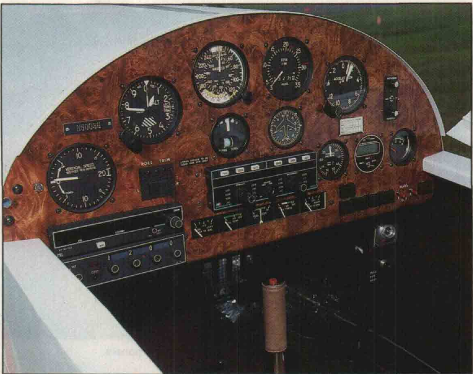
Today's standard sport aviation avionic package . . . a radio, transponder and loran.
