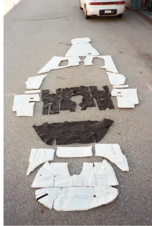
Twenty-one blankets are required for the whole aircraft. (Firewall in foreground to rear bulkhead in background.)
