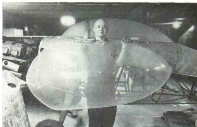
"Spare" canopy shown before windshield section is separated from rear canopy. \frac{1}{4} in. thick, type four, ultra-violet resistant plexiglass was used.
