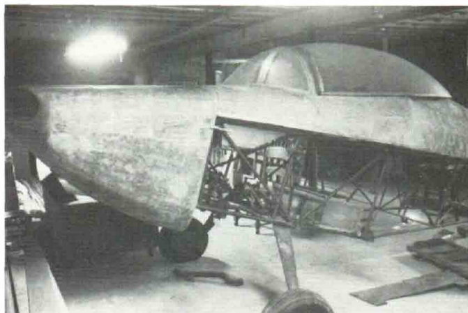
View showing symmetrical lines of fiberglass cowling and bubble canopy.
