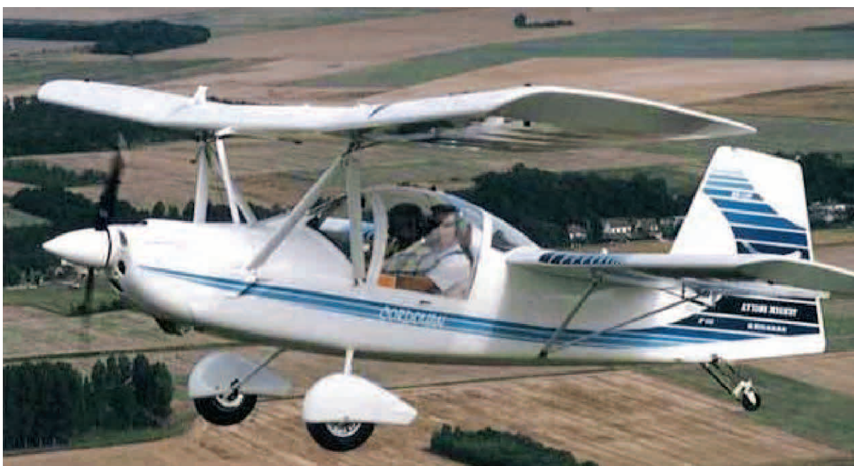
The HM-1100 CORDOUAN is the most recent design from the Mignet Aircraft Co. A true three-axis airplane, it has ailerons on the rear wing.
