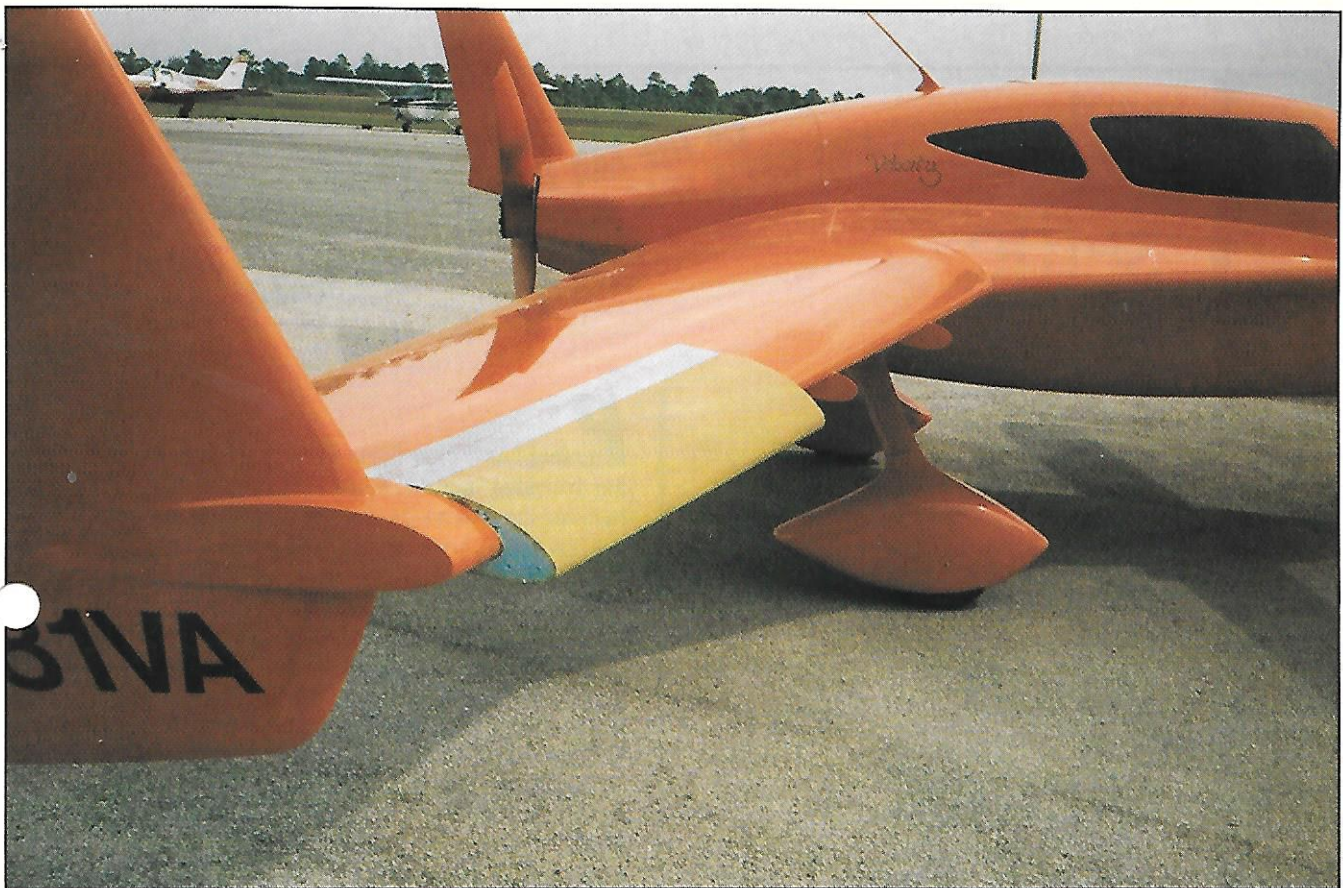
One of the cuffs tried on the original Velocity wing. A 60 inch cuff kept the airplane from getting into the deep stall condition and has been made available to builders of early kits. A new Velocity wing, now a part of kits, does not need the cuffs.
