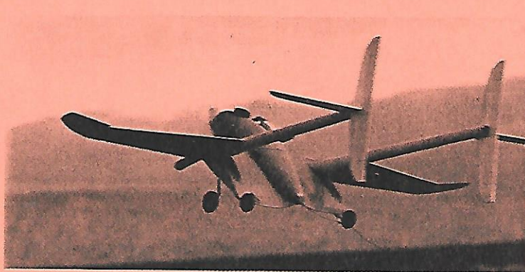
The Scorpion—a proof-of-concept model developed by Burt Rutan and Freewing Aircraft—climbs out. The photo shows the main wing and the tail booms angled in the same plane, both pointing into the relative wind.
