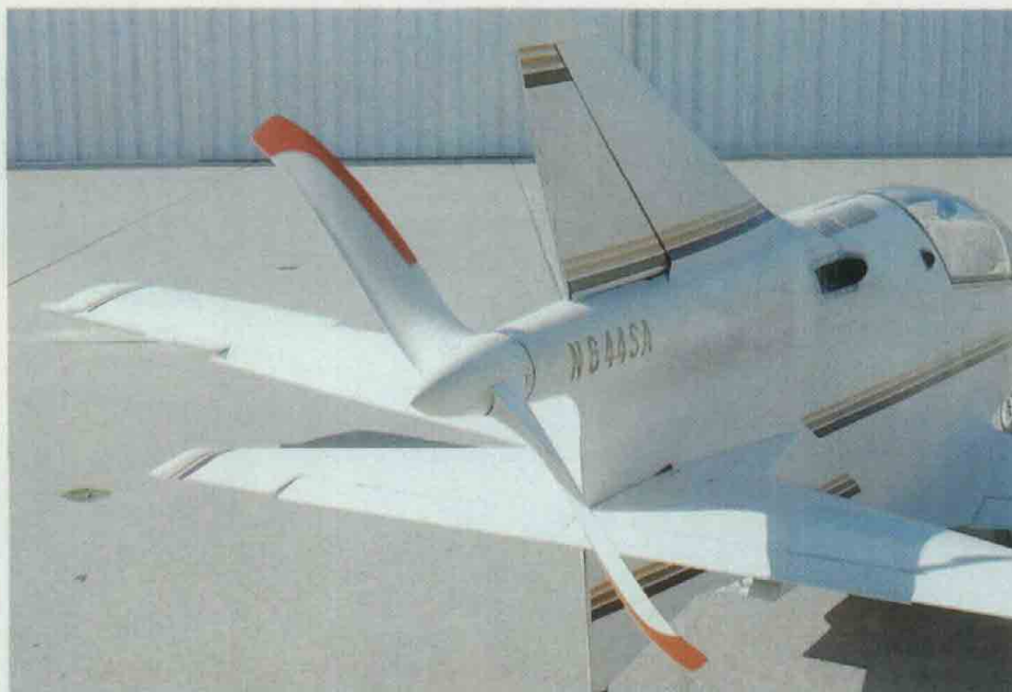
Photo Courtesy Seth Anderson Seth Anderson's specially designed propeller for the BD-5 — featuring a supercritical airfoil.
