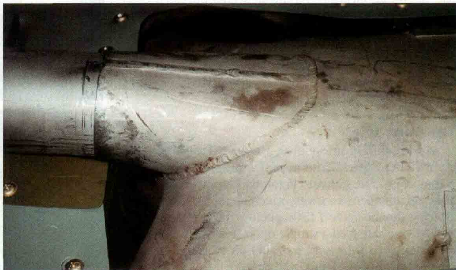
A P-38 NOS exhaust duct using OFW construction, lightly sandblasted, then passivated.
