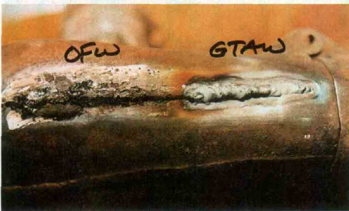
An old Wright collector ring welded with and without backup flux. Note the "sweat" on the top side of the flux weld. The root shows heavy "sugar" on the left side (I used filler on this weld), and on the right the flux cleans off leaving a bright finish. (No trick photography, just a graphic difference.)
