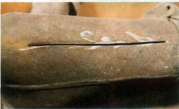
Rasty old exhaust tube gets the treatment: the saw kerf is welded using both methods.
