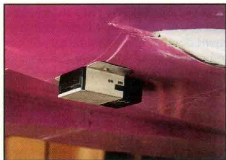
Flight engineer Chris Hawkins built this special mount to face the PropTach to the rear of the aircraft.
