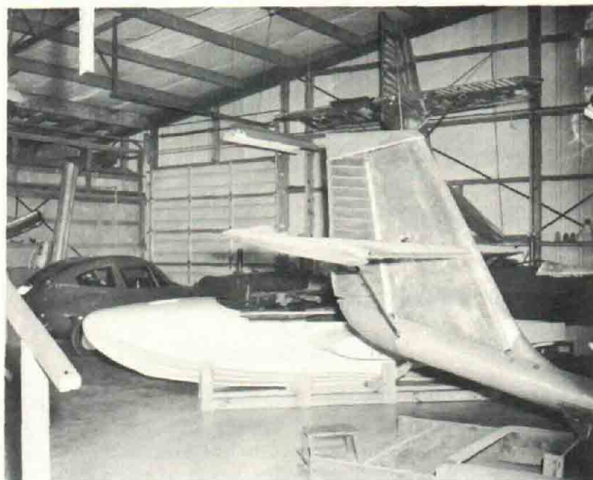
Two tail units for the Coot A are seen here, along with the prototype fiberglass hull shell for the Coot A.
