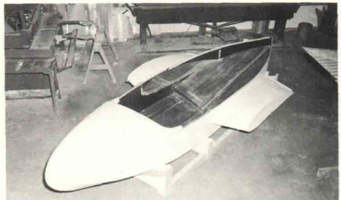
The Coot A fiberglass hull shell is to be offered to the builder in the near future. Stiffeners and frames would have to be installed according to the drawings. Neither the Coot A nor the Coot B will lend themselves to a four-place arrangement.
