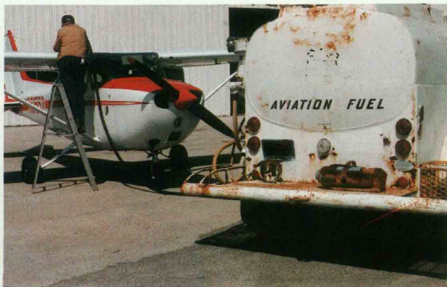
If the fuel truck is grimy, dirty and rusty, what is the condition of its contents? Although the truck is marked aviation fuel the type or grade of fuel is not indicated. Note the rusty disintegrating cylinder on the back bumper. That's a fire extinguisher!
