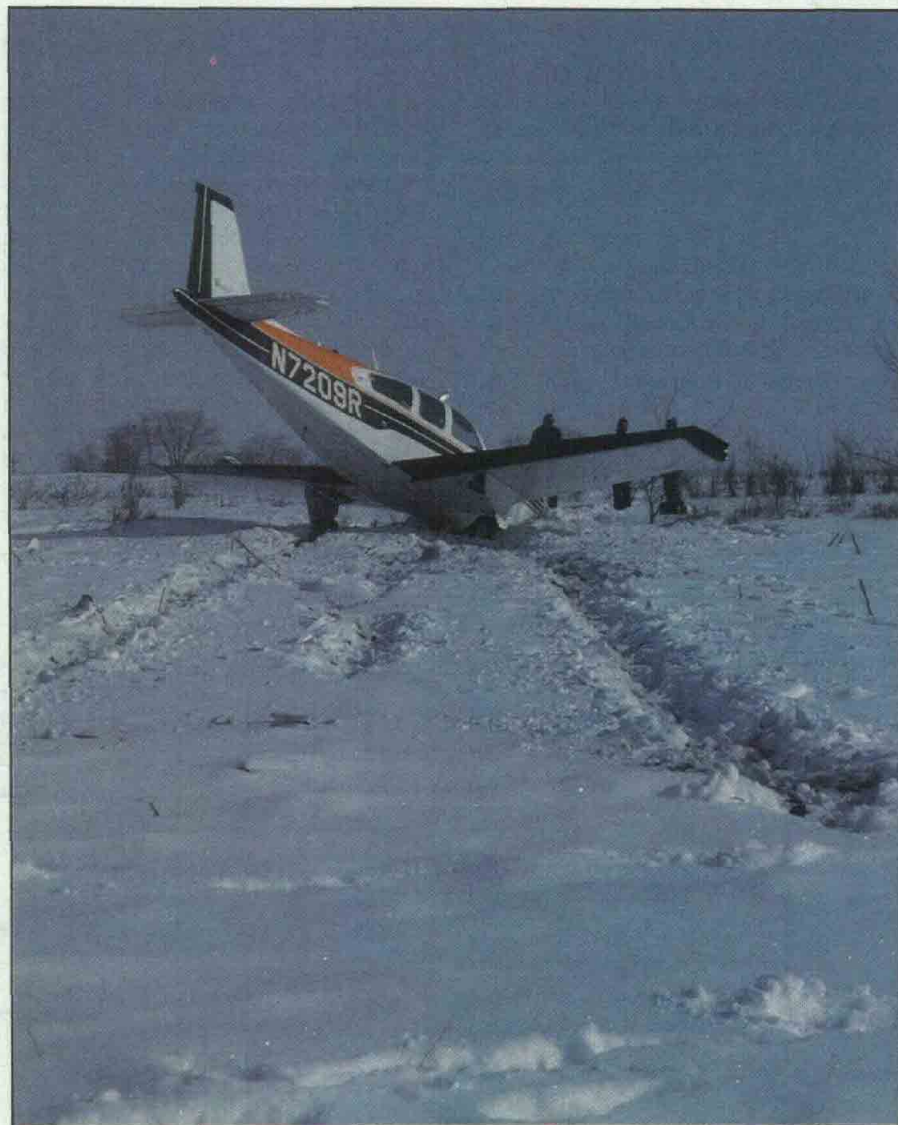
Result of fuel cut off is a forced landing just off the end of the runway by this Beechcraft A-36.
