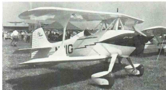
Fine finish possible with fabric covering adds to performance.
