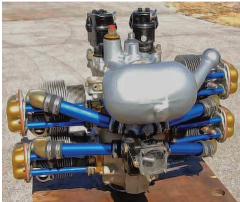
Underside of a recently overhauled A80. Differences between A-series models are not generally distinguishable by cursory examination. Kidney-shaped oil sump identifies the series.
