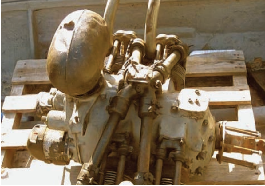
A typical core engine as found in barns, shops, hangars, warehouses, and hanging on abandoned aircraft. This one is an A65 and was sold in "as-is-where-is" condition from an abandoned freight liquidator for $250. Dented oil sump is very common but can be corrected by pressurizing the sump with compressed air and gently heating the dented area with a torch until the dent is blown out.
