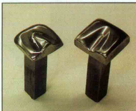
This is a special set of "thumb nail" dies made for the Pullmax to allow it to shrink sheet metal panels.
