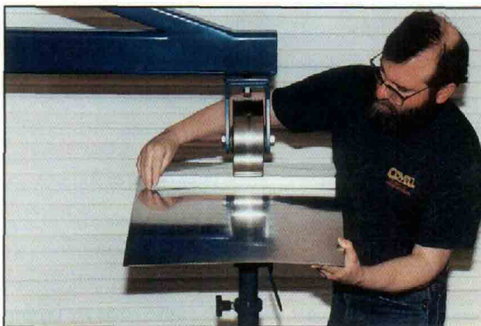
You can see there is crown both right to left and front to back on this panel. This has resulted from about two minutes of wheeling time. Note how glassy smooth the surface is.
