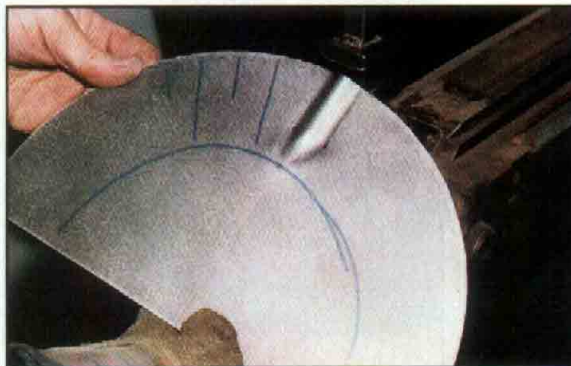
This is a special set of "thumb nail" dies made for the Pullmax to allow it to shrink sheet metal panels.
