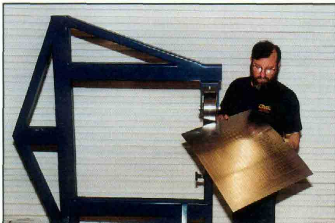
In this shot you can faintly see the tracks left by the wheels. The tracks are so close they almost touch. The more uniform you can maintain your tracking pattern, the smoother the panel will stay while being shaped.
