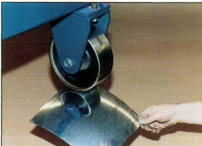
Here is a smaller panel being shaped with a higher-crown wheel. There is about 80 pounds of pressure between the upper and lower wheels, and it is quite easy to roll the sheet metal between them.
