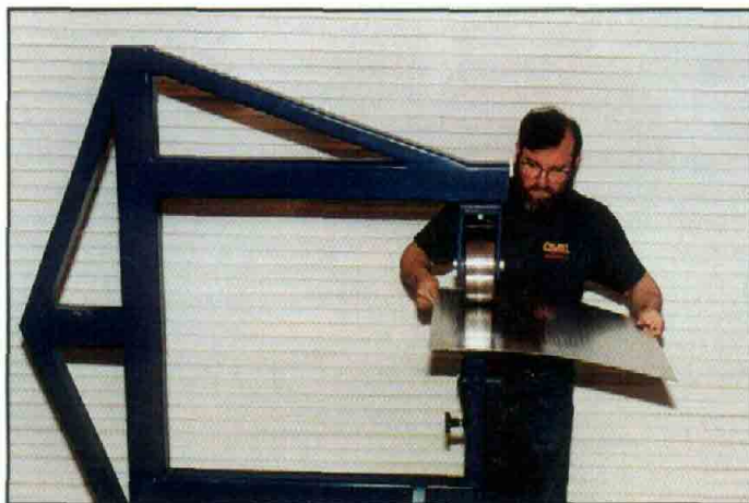
This is a modern, fabricated frame wheeling machine, being used with a low crown lower wheel to put a very slight compound curve in a sheet of aluminum about two feet square.
