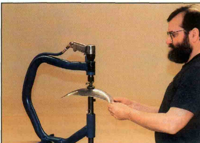
This is a pneumatic planishing hammer, being used to smooth a small domed panel originally roughed out with a mallet and sandbag.
