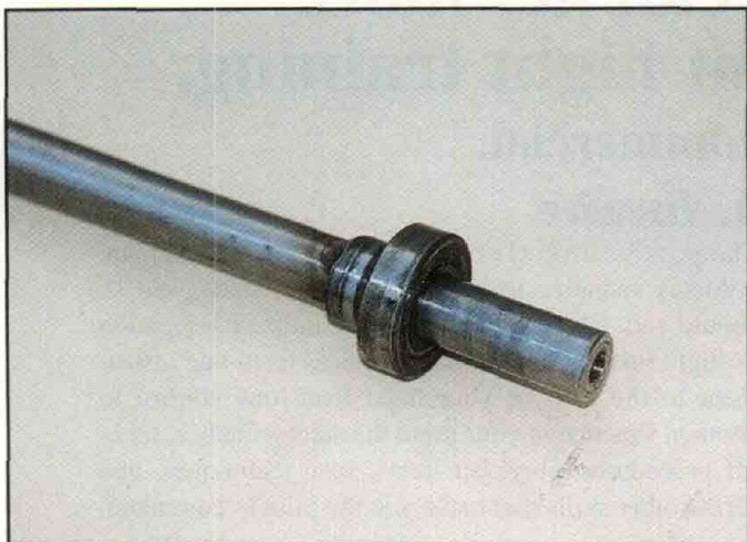
The roller end of the main shaft has a collar welded in place. The top roller is clamped against that stop through the inner bearing race by spacers and the bolt in the end of the rod.
