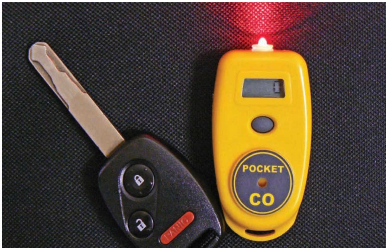
The Pocket CO 300 carbon monoxide detector, about the size of an average car key, continuously displays CO levels, and a flashing LED indicates the device is operating.
