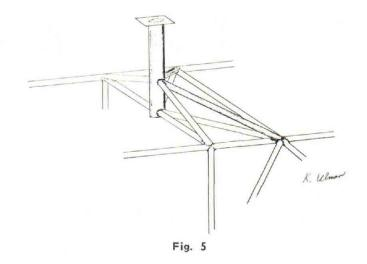
structure slightly modified with the addition of two lateral brace tubes and a single tube pylon.
