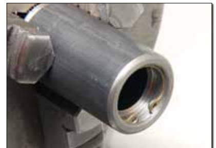
Turning a groove and testing the fit of a \frac{3}{4} -inch internal snap ring.
