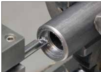
Turning a groove and testing the fit of a \frac{3}{4} -inch internal snap ring.
