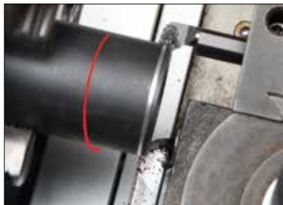
(Left) Turning an external groove with the Micro 100 tool. Note the spindle rotation is clockwise. (Right) Testing the fit of a 1-inch external snap ring.
