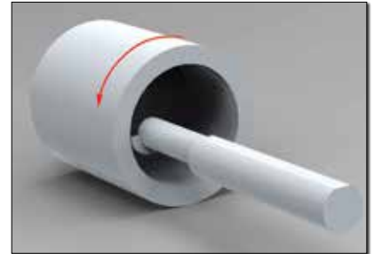
Illustrating the tool position and spindle rotation for using a bore grooving tool for both outside (left) and inside (right) grooving.
