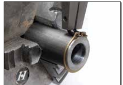
(Left) Turning an external groove with the Micro 100 tool. Note the spindle rotation is clockwise. (Right) Testing the fit of a 1-inch external snap ring.
