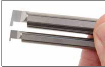
Micro 100 solid carbide retaining ring grooving tools. The top tool makes a groove 0.064 inch wide and the bottom makes a groove 0.030 inch wide.
