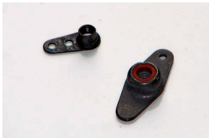
Two types of locking nut plates. The left one uses out-of-round threads; the right one uses standard Nylok.
