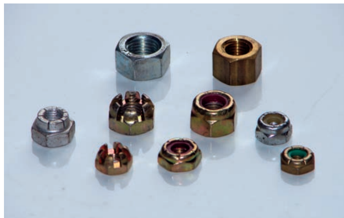
Front: Locking castellated nut (for high-temperature installations), castellated AN nuts, and standard AN365 (taller) and shear nuts. Back: For special applications: plain nut and brass exhaust-mounting nut.
